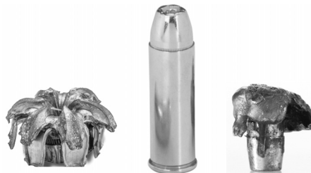
When bullets hit their targets, the soft lead deforms. The high-performance, expensive, bullet on the left has “opened up” almost perfectly.
