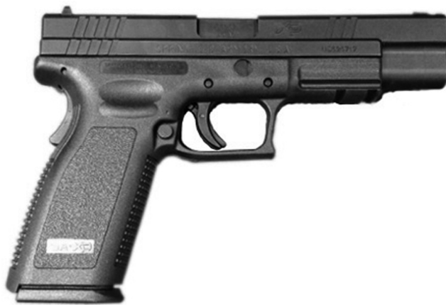
The frame of this pistol is made from plastic polymers. Note the double trigger, a safety mechanism on some modern pistols. The forward trigger is a safety. The rear trigger operates the gun like a standard trigger. To fire the gun, the shooter presses both triggers in one continuous motion.
