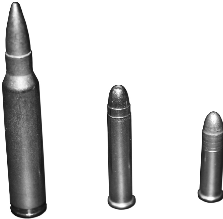
Different types of ammunition. From left to right, .223 Remington, .22 WMR, and .22 LR. Note that the bullet (the top part) for the .223 Remington is only 3/1000 of an inch wider than the .22 caliber bullets. But the .223 Remington's case is much wider and larger, allowing more room for gun powder, making it far more powerful than the other two.
