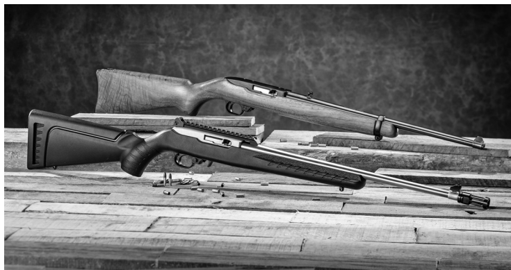
A pair of .22 caliber semi-automatic rifles. This is the same gun, in two different configurations. The one in back has a traditional wood stock, the one in front has a modern plastic polymer stock. The black gun also has a rail, onto which a scope can be mounted, and it is a muzzle brake (mounted on the muzzle) which stabilizes barrel vibration, so that the user can stay on target for the second shot.
