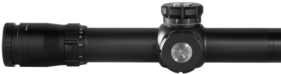
In this rifle scope, the dial on the left is used to adjust magnification, from 2X up to 15X. The two dials on the right are used to make small vertical and horizontal adjustments, so that the center of the scope points exactly to the barrel's point of aim. The scope can be attached to a rifle by a pair of mounting rings on the top of the rifle (not shown).
